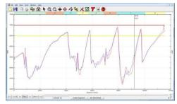
Evaluating RPM data can be used to evaluate engine performance. Gearing, shift time, and engine acceleration curves are commonly evaluated to improve the racecars performance as well as reduce the potential wear on your equipment.
